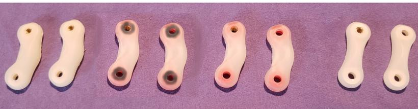
In a matter of minutes, the hinges in the AFO shown at right can be replaced to modify the device's stiffness, and to change its behavior from neutral to dorsiflexion assist.
